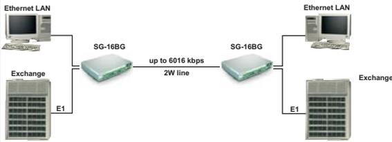
Connect two LANs and two digital branch exchanges via the same 2W pair.
