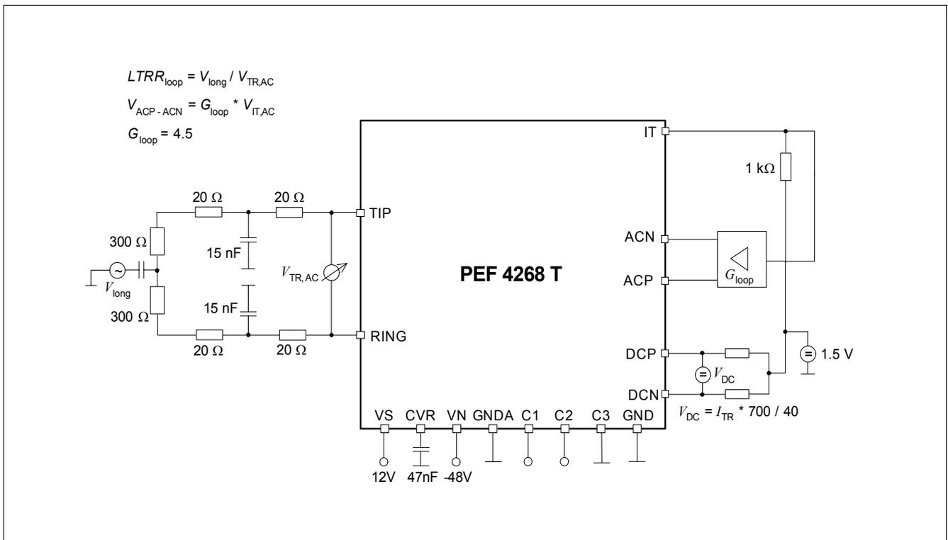
Figure 13 Longitudinal to Transversal Rejection Loop
