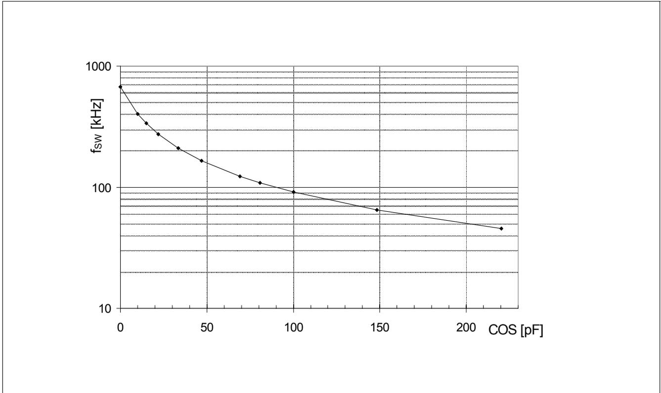
Figure 11 Oscillator Frequency vs. Capacitance at COS
