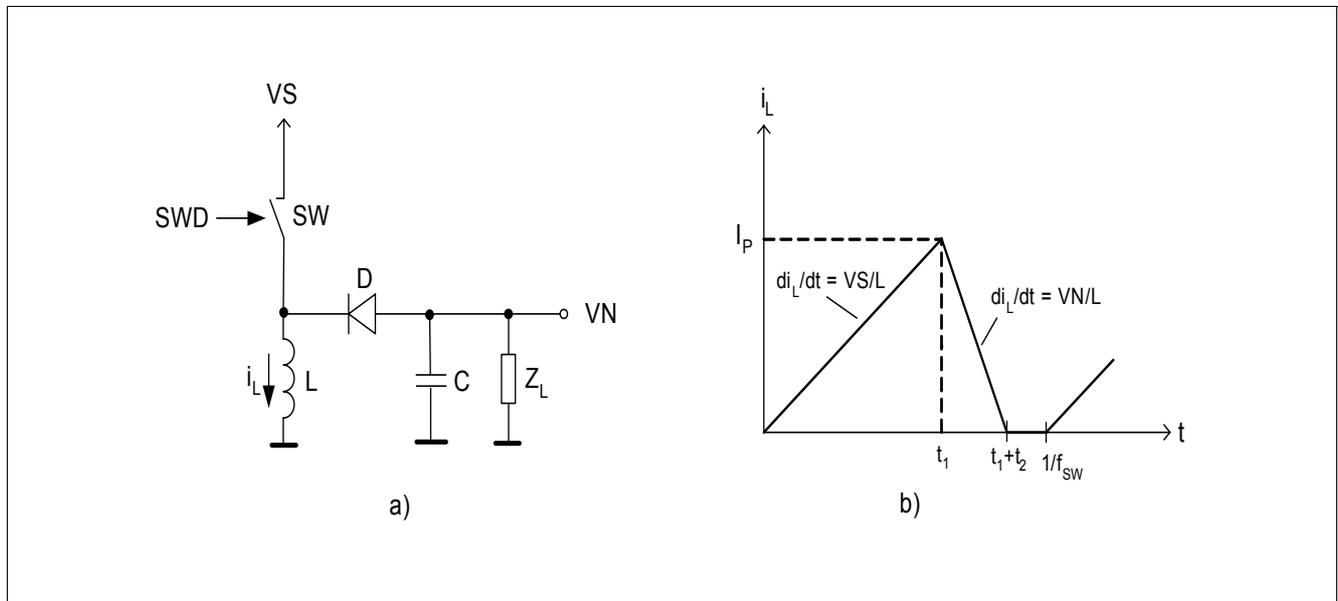
**Figure 7 Basic Buck-Boost Topology (a) and Inductor Current (b)**
