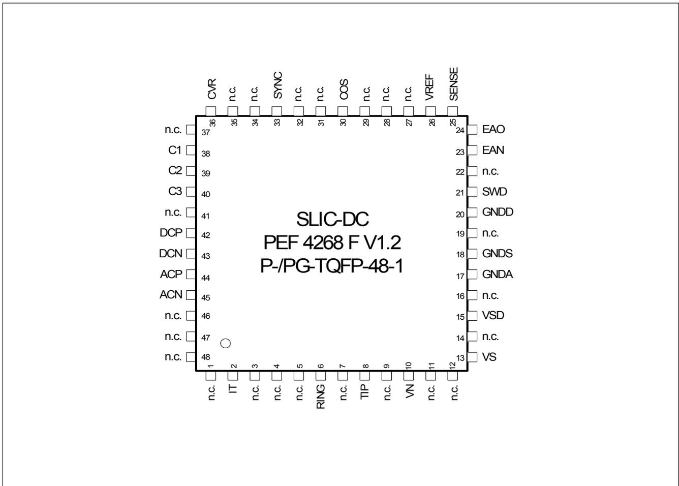
Figure 2 Pin Configuration P-/PG-TQFP-48-1 Package (Top View)
