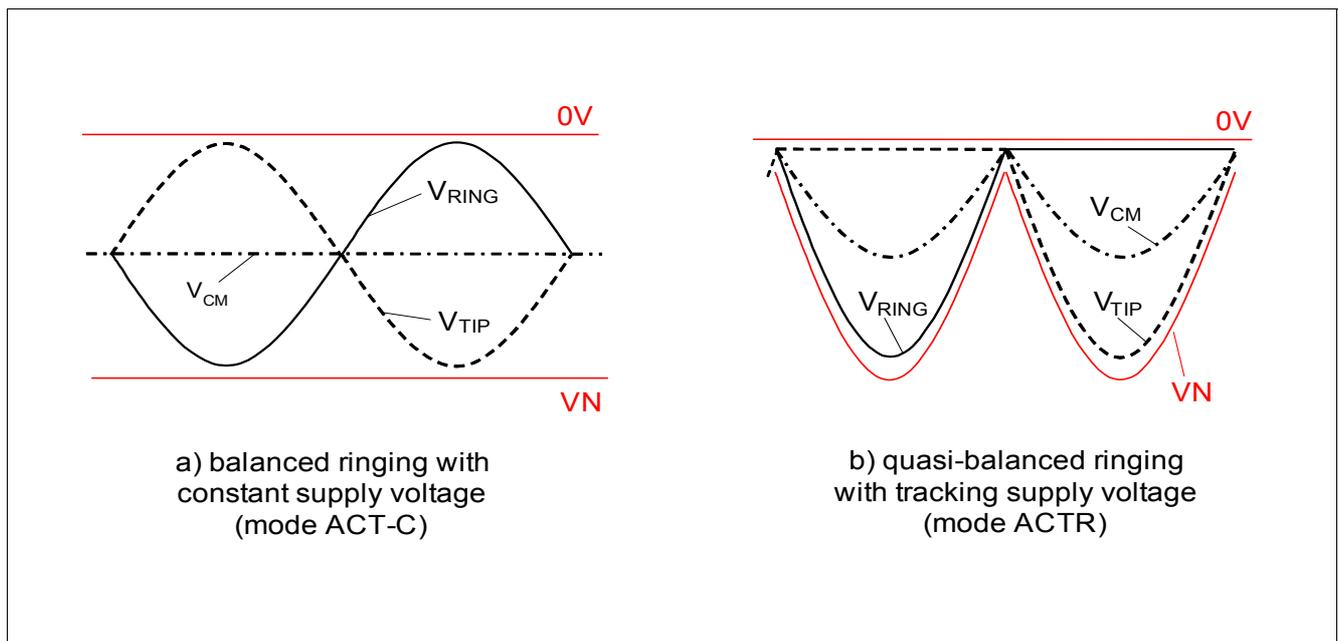
Figure 5 Comparison of Ringing Waveforms
