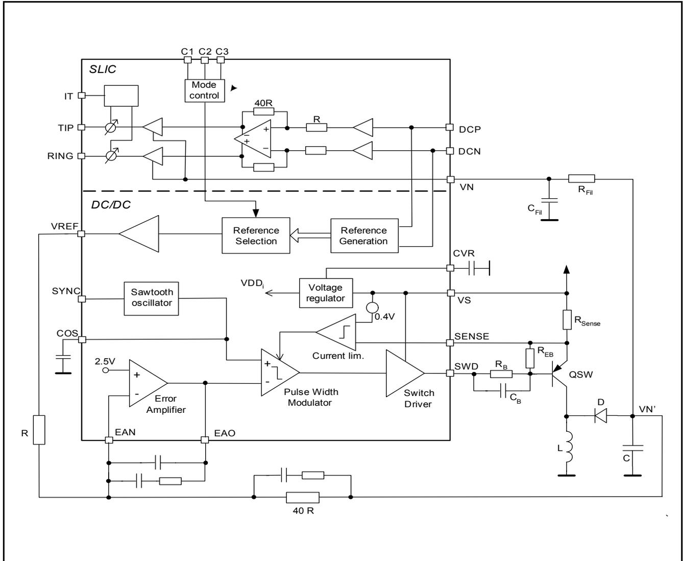
Figure 8 DC/DC Blocks and Components
