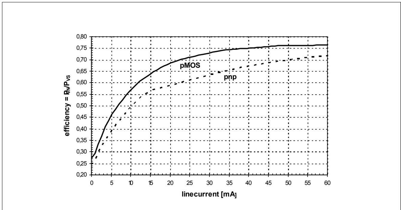
Figure 9 Efficiency versus Line Current,  $f_{sw} = 105 \text{ kHz}$
