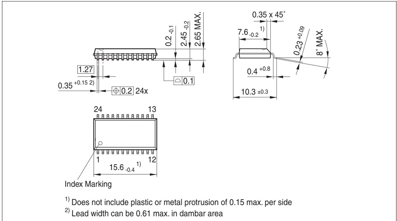
**Figure 14 P-/PG-DSO-24-8** (Plastic/Plastic Green Dual Small Outline Package)
