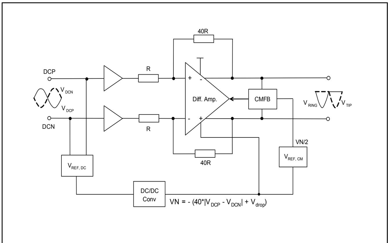
Figure 6 Generation of Quasi-balanced Ring Signal
