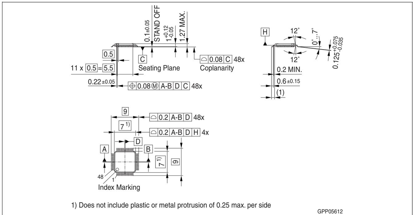
**Figure 15 P-/PG-TQFP-48-1** (Plastic/Plastic Green Thin Quad Flat Package)
