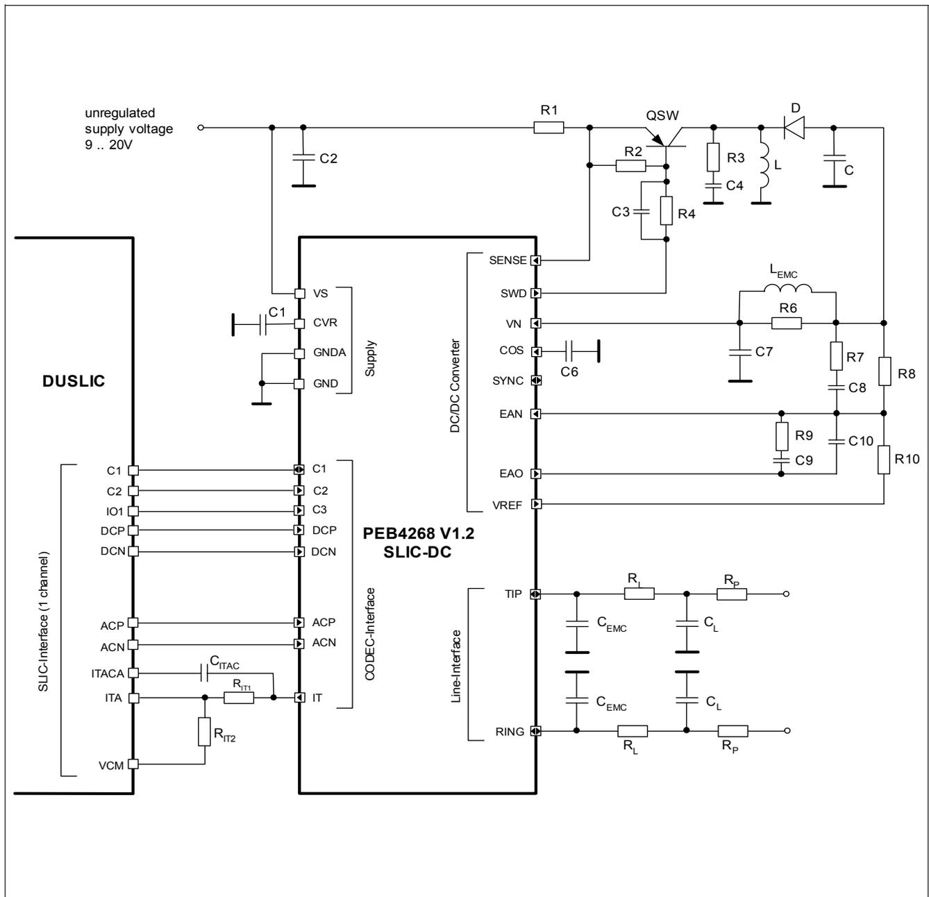
**Figure 10 Application Circuit**
