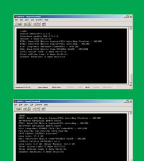
Management software allows define operation modes for each interface, collect statictics for each interface, make use test mode to determine error rate of the line, do configuring of the remote modem. Anyway customer can flexibly share SHDSL channel bandwidth among interfaces in use. Step size is 64 kbps for each interface.
