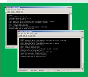
Management software allows define operation modes for each interface, collect statistics for each interface, make use test mode to determineerror rate of the line, do configuring of the remote modem. In any casecustomer can flexibly share SHDSL channel bandwidth among interfaces in use. Step size is 64 kbps for each interface
